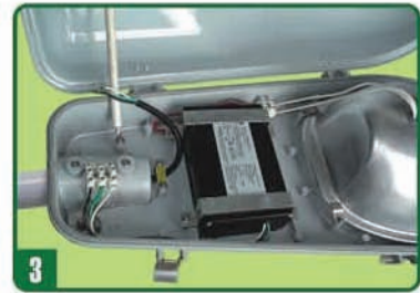
3 Assemble the pole with the fixture. Adjust the level and tighten the set screw with the torque at 13-15NM.
