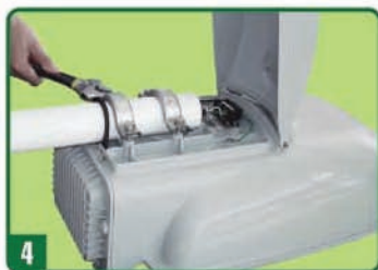
4 Set the level of the fixture and tighten the bolt at the torque of 13~15 N·M.
