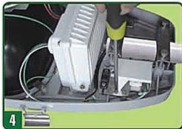
4 Loosen the screw and remove the hood of wiring box and top cover of wiring press.
