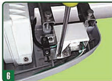
6 Assemble the wiring box and fasten it with the screw.
