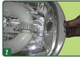
2 Loosen the steel clip
