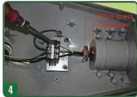
4 Pull the customer's cable through the grommet and wire press. Connect it to the terminal correctly.
