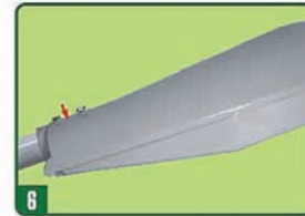
6 Adjust the angle of the fixture and fasten the hex bolt M10×35 with torque at 13~15 N·M, correctly.
