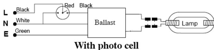
NOTE: Efficient and reliable grounding is necessary for personal safety and the proper use and operation of the electronic ballast to meet EMC standards without interference to the equipment. Do not use this luminaire without proper grounding.
