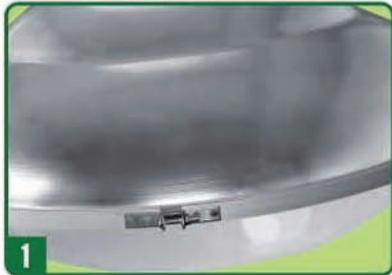
Put the cover on the hood. Assemble the hood and cover in the groove of the ring and fasten with  $\pm$  headed screw M4X25 and nut M4. Check that the long side of the ring shall be at the cover side.
