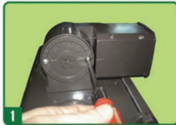
1 Unscrew the screw of the cover of the splitfitter and remove the cover.
