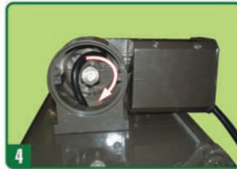
4 Pull the cable through the fixture. Set the angle and fasten the split fitter with the hex bolt.
