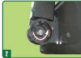
2 Unscrew the hex bolt of the split fitter.
